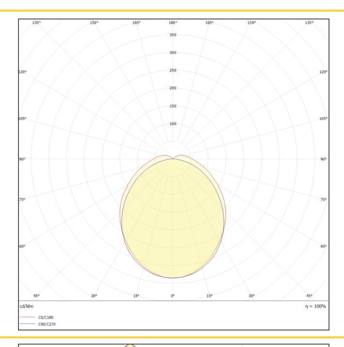
36 Watt 110° Beam Angle Cone Diagram
